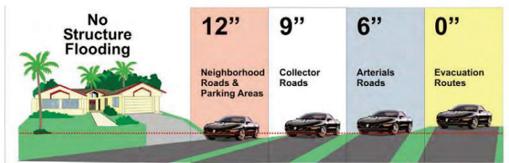
Figure 4-1 Acceptable Flooding for a 100-Year Storm
